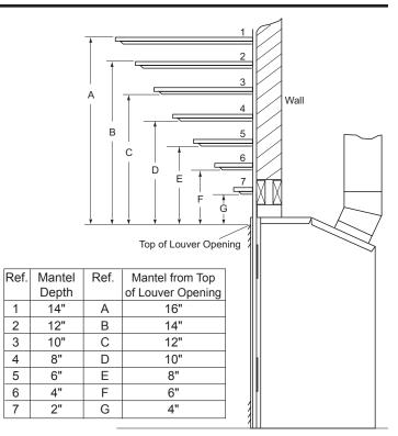
Figure 6 - Clearances for Combustible Mantels
